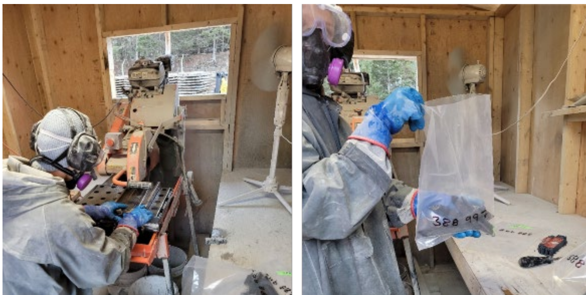
Figure 11-1: Mechanical drill saw with pre-marked sample bags
