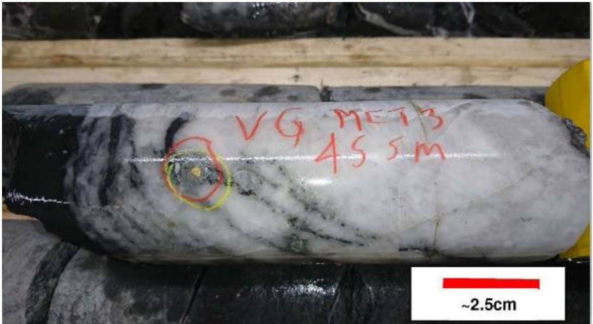
Figure 7-6: Visible gold in graphitic argillite: Hole BR-17-03.
