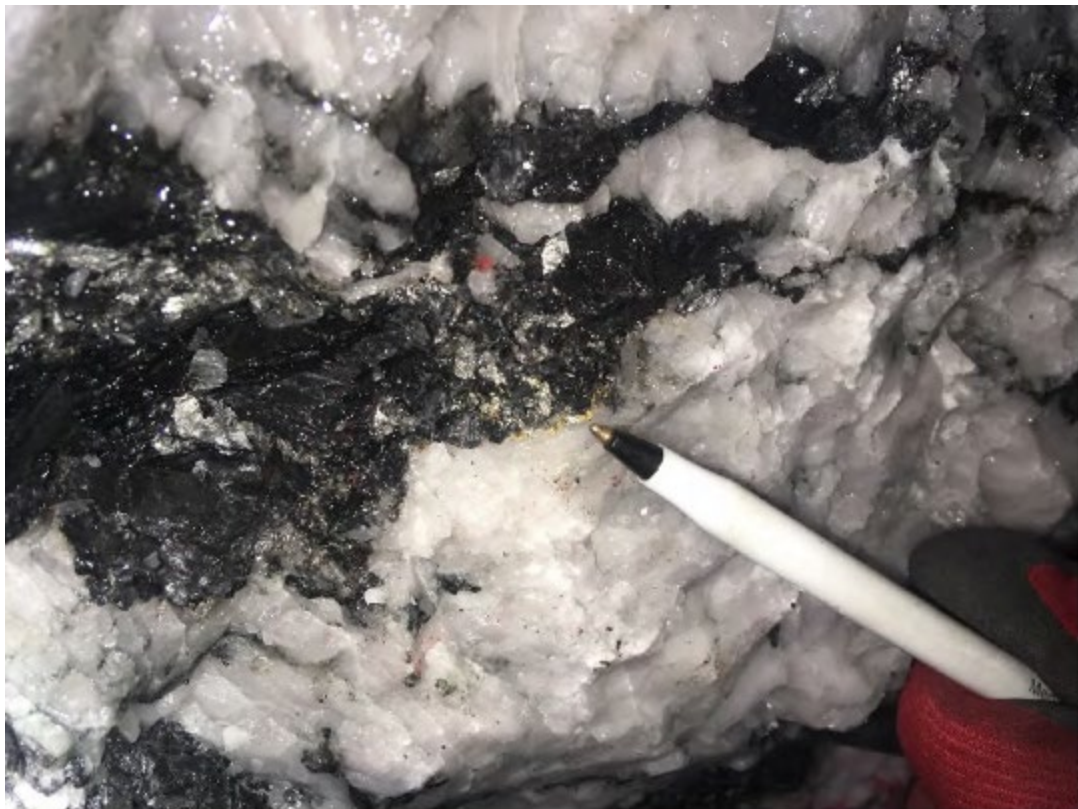
Figure 6-5: Visible gold along margin of quartz vein-argillite contact in Level 3 East Round 3
