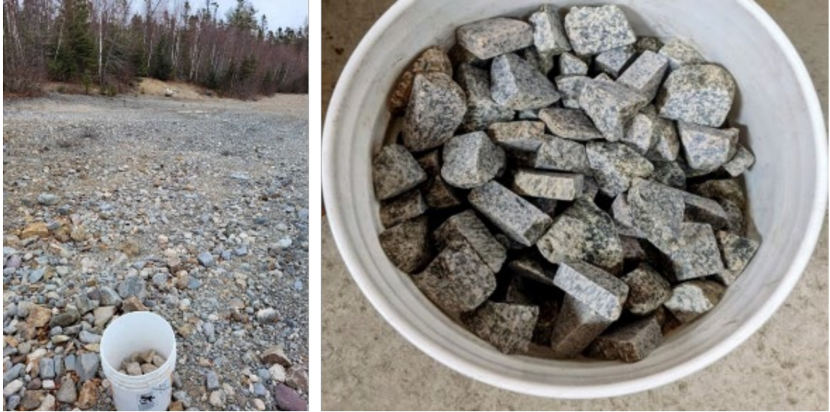
Figure 12-14: Blank material from granite boulder rock quarry in Stormont, Nova Scotia
