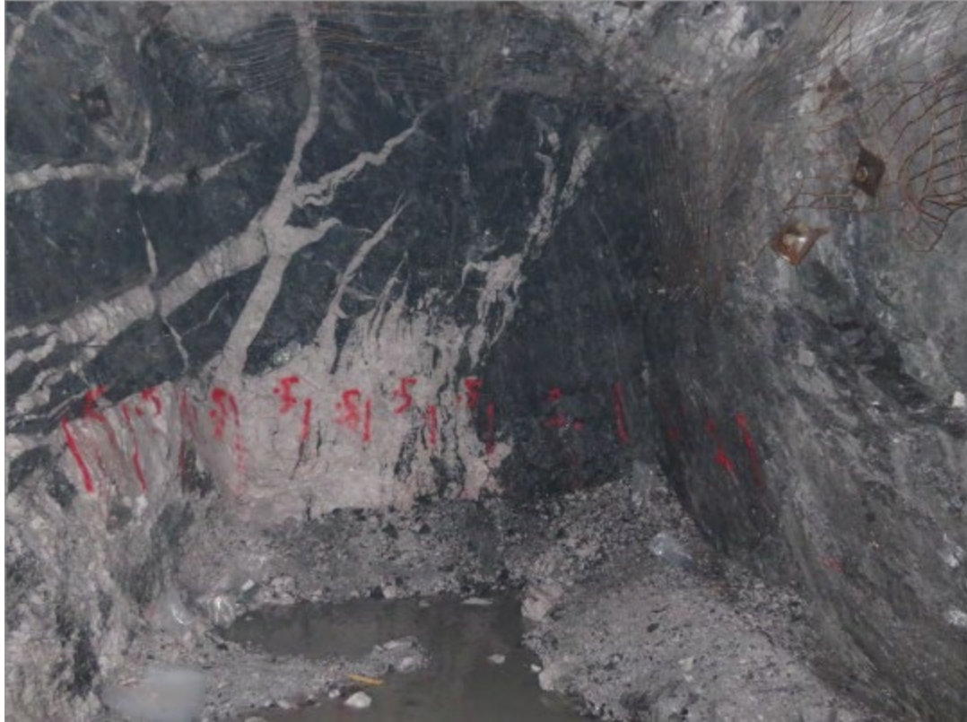
Figure 6-2: Level 1 West Round 1 - thin argillite-quartz veins adjacent to extensional quartz veins (looking west)
