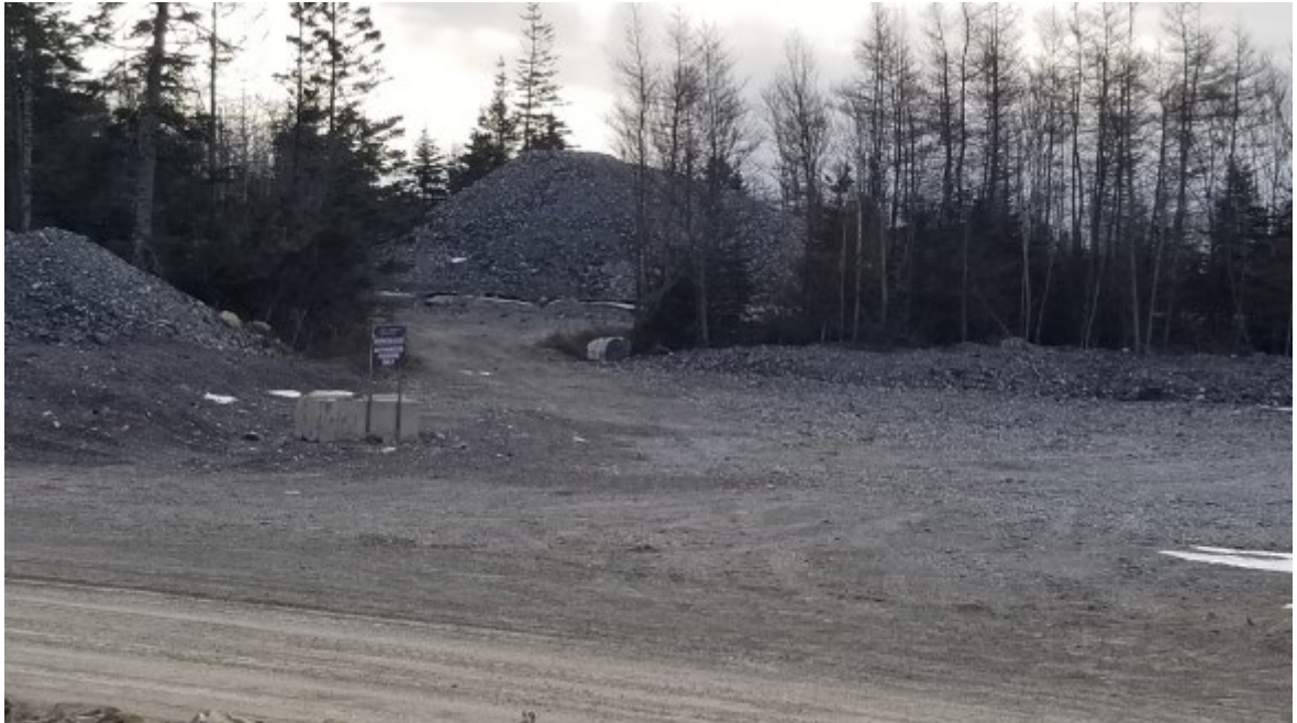
Figure 12-17: Onsite mineralized stockpile
