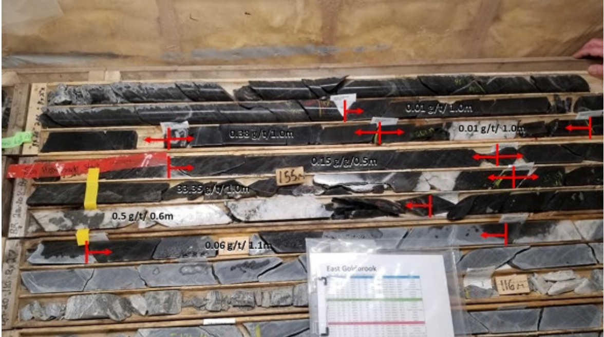
Figure 12-10: QP selection of core samples for review of assays results over larger areas and to test local variability
