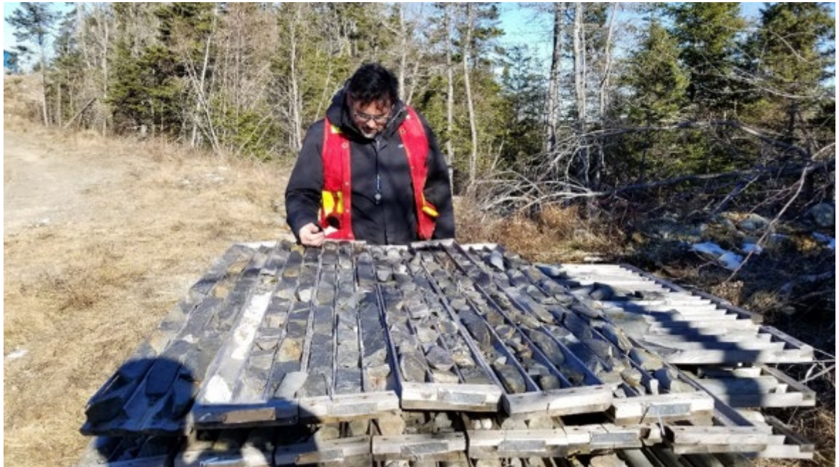
Figure 12-8: Historical Company core being reboxed and moved into the current storage facility
