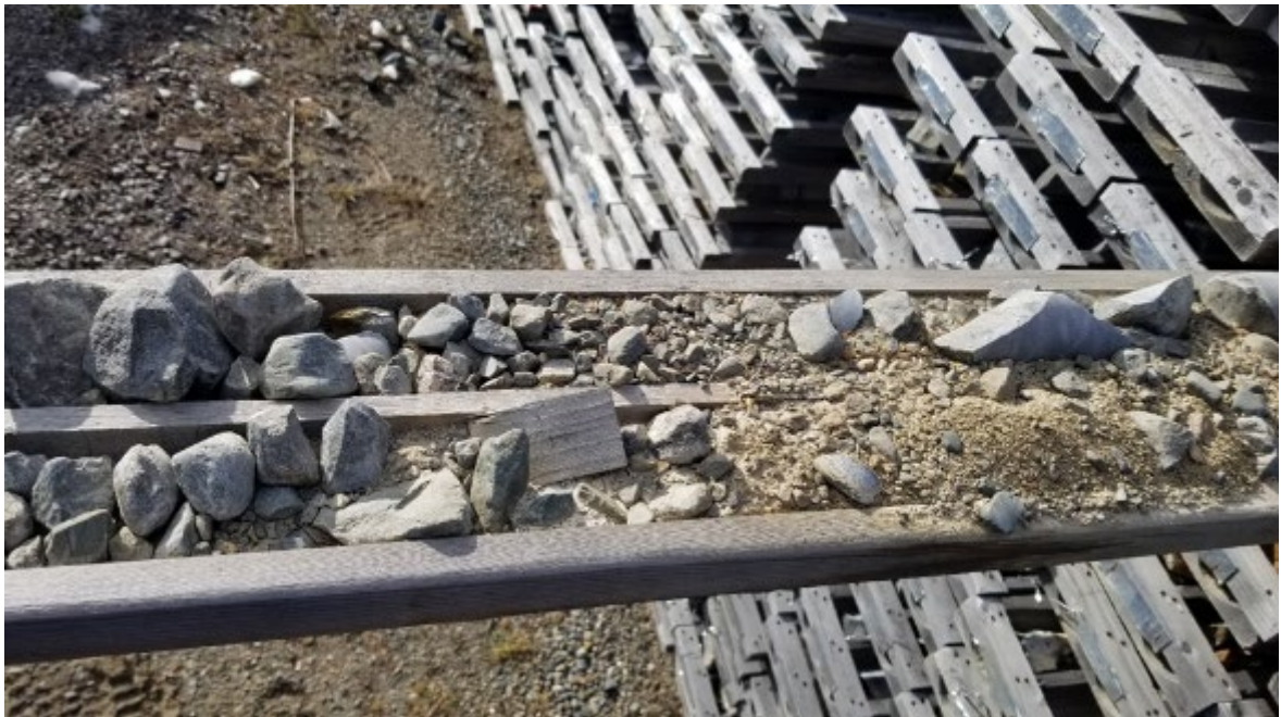
Figure 12-19: Hole BR-17-05 in the vicinity of the underground portal displaying similar overburden material to what is located within the underground portal area.
