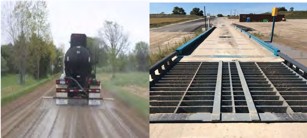
Figure 1 Water Truck* (left) and Grizzly Screen (right)
