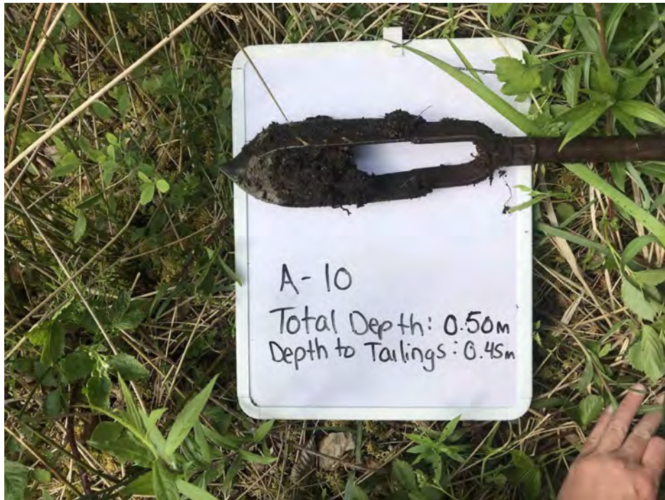
PHOTO 3 - SOIL SAMPLE WITH TAILINGS PRESENT AT DELINEATION POINT A-10
