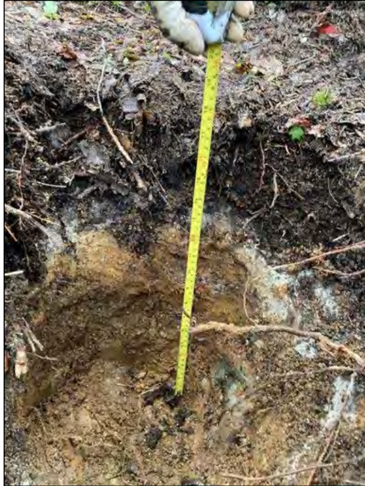
Figure 2-2: Example of an overburden test pit (LXGB-2021-TMFOB-02) displaying distinct organics (top, dark) and till (beige) horizons.
